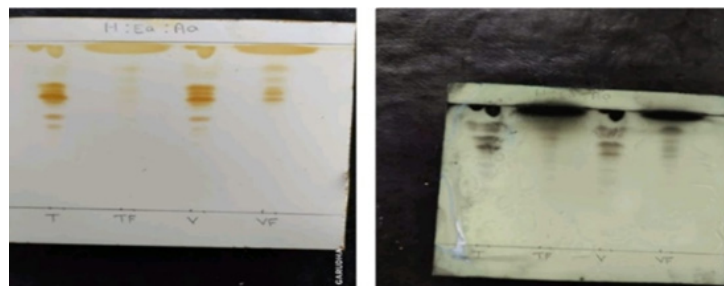
Figure 2: TLC of Fixed Oil in Iodine Chamber
